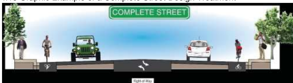
Figure 4.15 Graphic Example of a Complete Street Design Treatment
