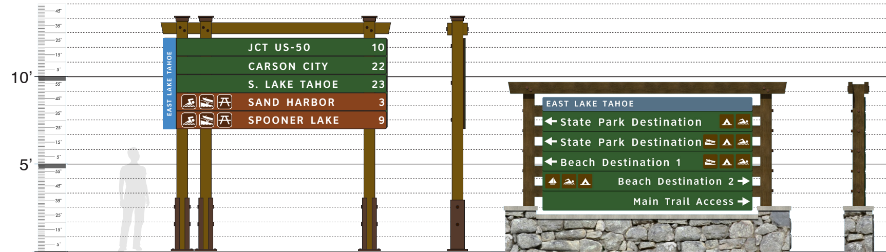
Sign Type A Vehicular Pole-Mounted Directional
