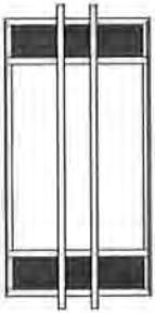
TWO HORIZONTAL & TWO PROUD EXTENDED VERTICAL TRIM BARS W/ SOLID ENDS (2HTB/2PEVTB/SE)
