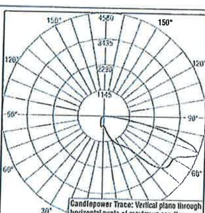
Independent Testing Laboratories certified test. Report No. ITL64565. Candlepower trace of 6000K, 120 LED Type III Medium area luminaire with backlight control and 7,023 initial delivered lumens operating at 350mA. All published luminaire photometric testing performed to IESNA LM-79-08 standards.
