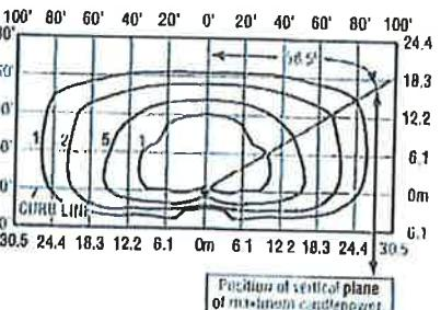
Isofootcandle plot of 6000K, 120 LED Type III Medium area luminaire with backlight control at 25' A.F.G. Luminaire with 7,419 initial delivered lumens operating at 350mA. Initial FC at grade.
