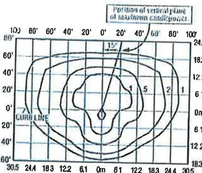
Isofootcandle plot of 6000K, 120 LED Type III Medium area luminaire at 25' A.F.G. Luminaire with 9,093 initial delivered lumens operating at 350mA. Initial FC at grade.
