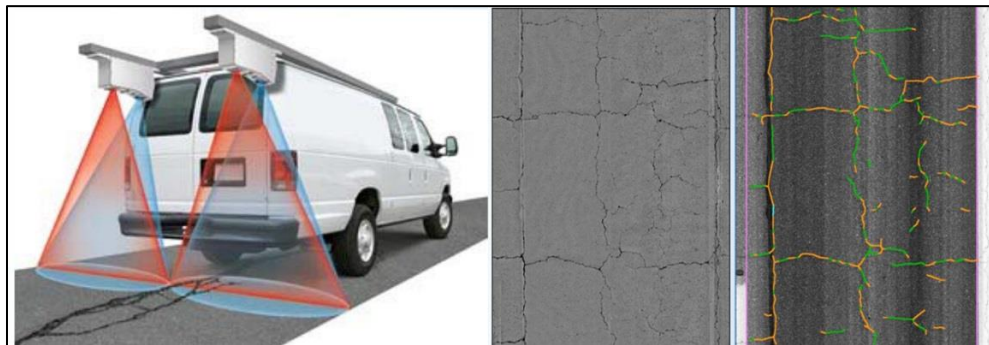
Figure 3 Schematic of LCMS 3-D Operation – Collection, Range Imagery and Crack Detection
