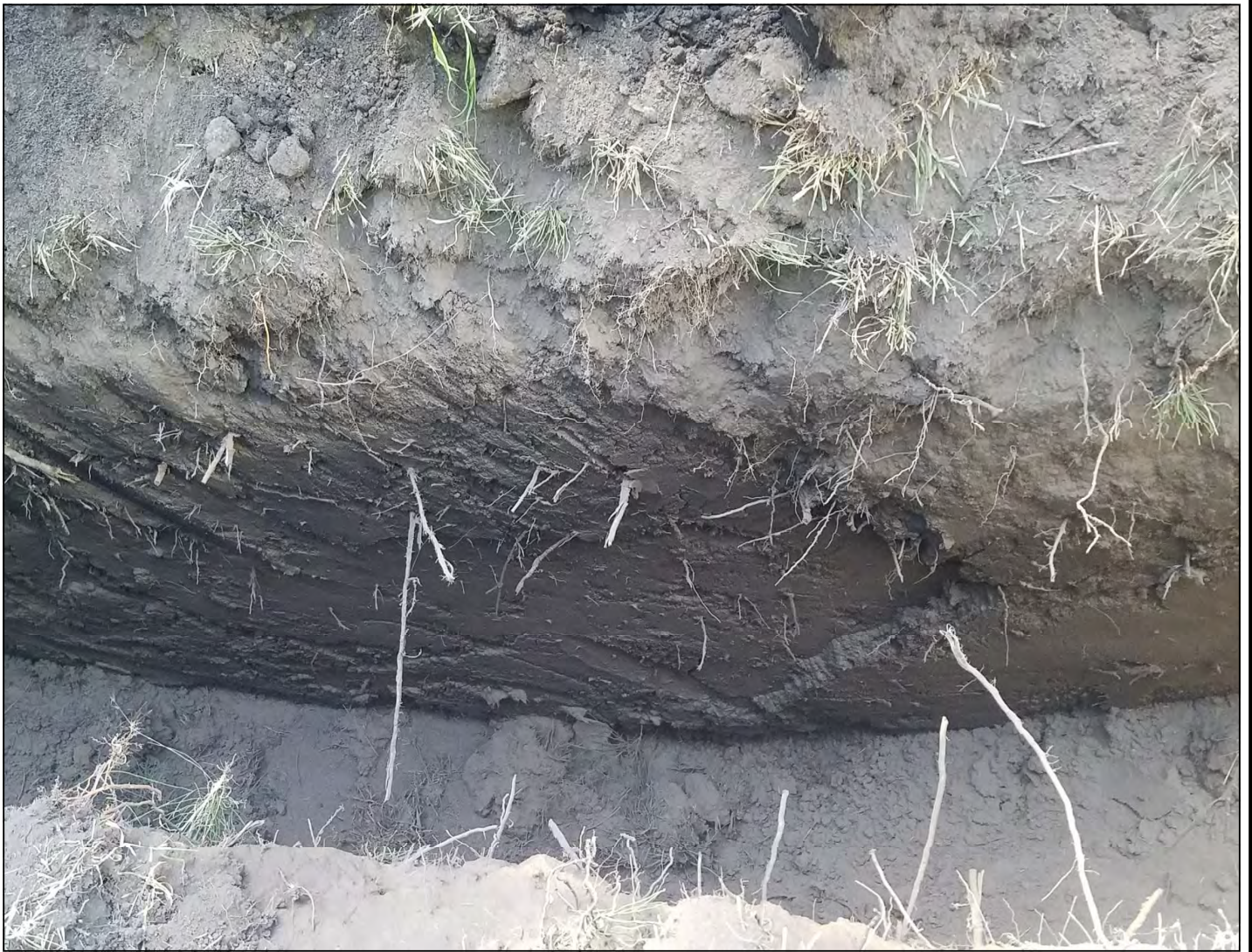
Figure 2: West side of fault trench. Upper 1' is lighter brown silty sand and lower 5' is dark brown silty sand with roots throughout. Right side of sidewall shows a lighter color, that is just sunlight shining through the trees.
