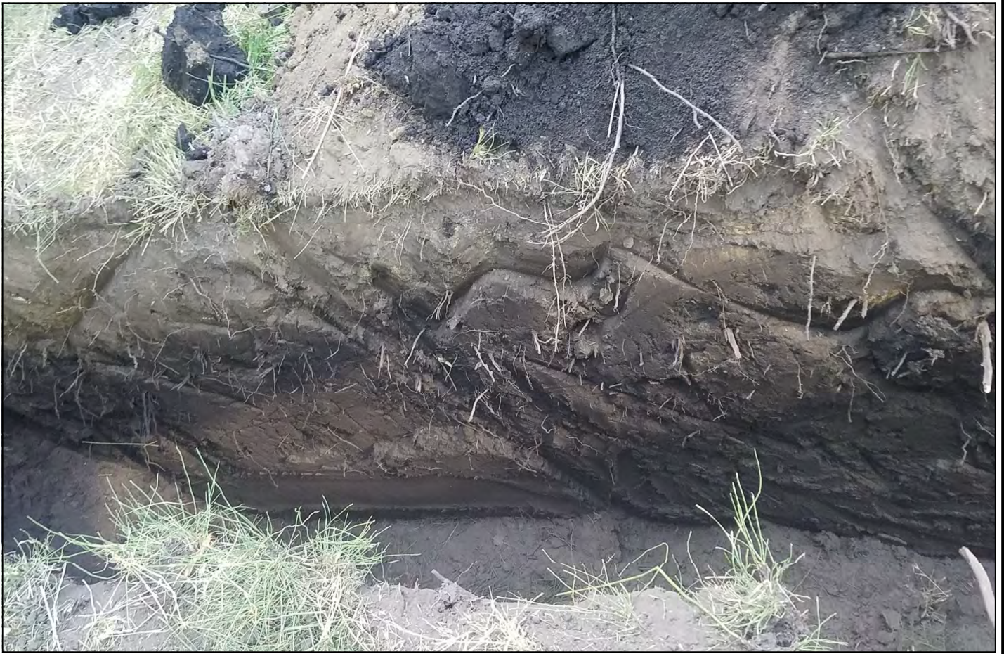
Figure 1: East end of fault trench, shows the surface going down hill. Upper 1' is lighter brown silty sand and lower 5' is dark brown silty sand with roots throughout. Middle of sidewall shows a lighter color, that is just sunlight shining through the trees.
