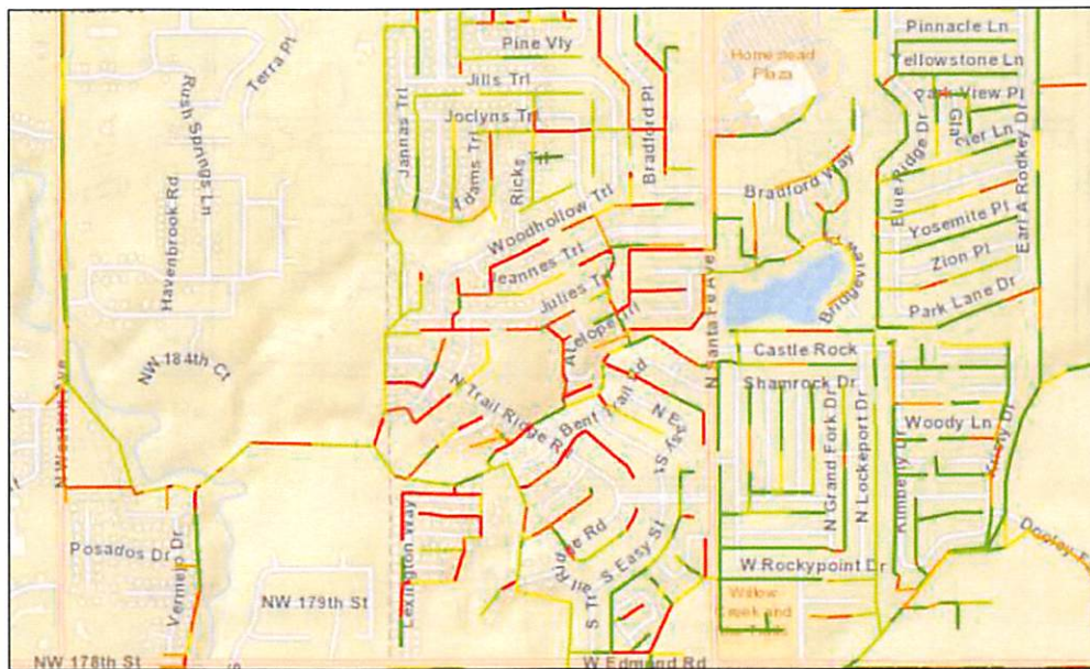
Figure 8: Example of sewer system broken up from manhole to manhole; Green to Red symbolizes Good to Poor condition.
