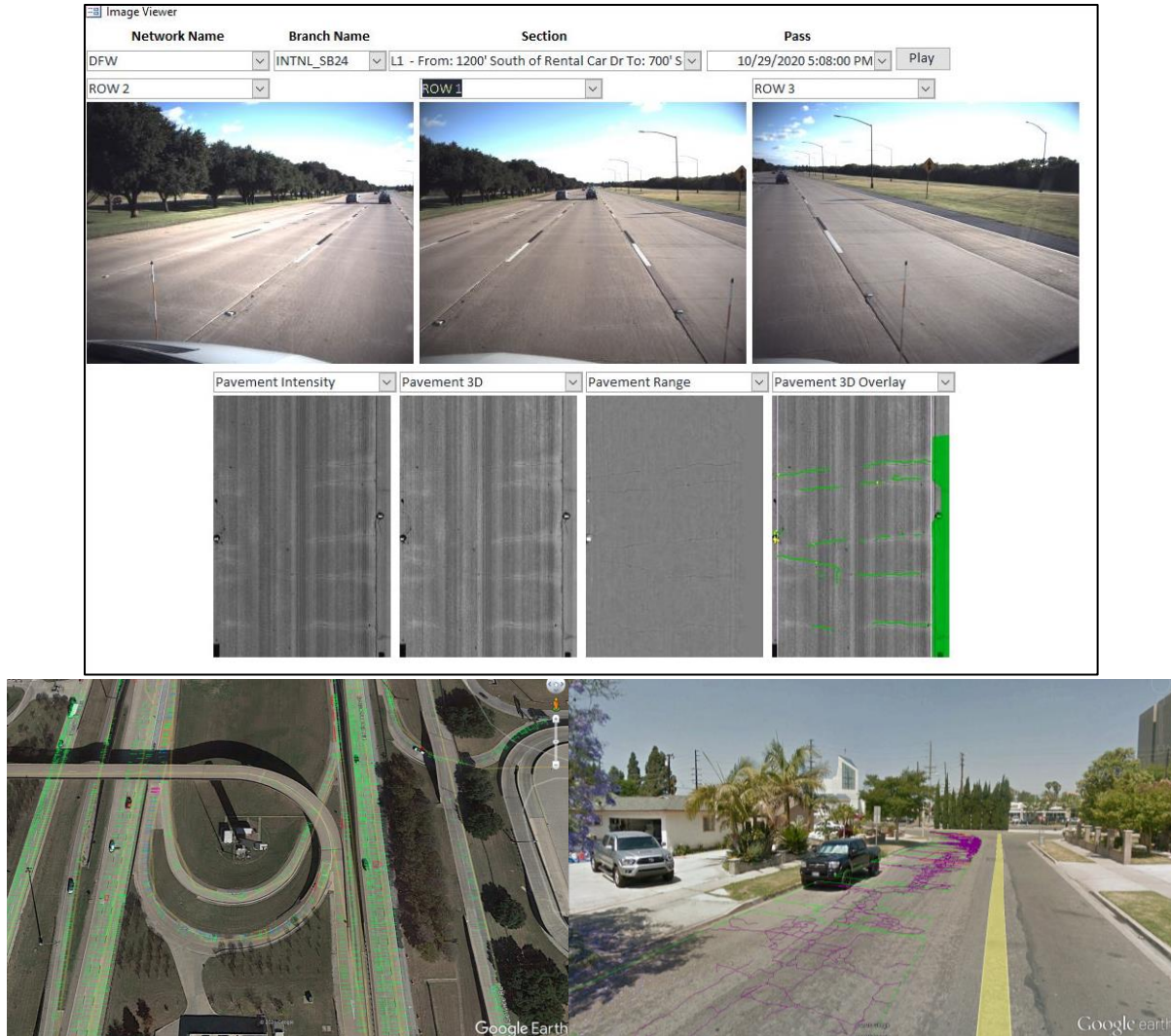
Figure 2 — ARA Right-of-Way Image Viewer and Google Earth Crack Map.
