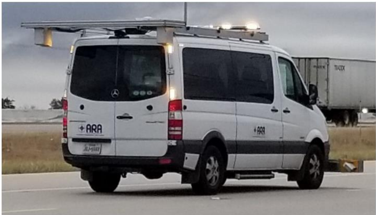
Figure 1 — ARA Multi-Function Vehicle (Equipped with 3-D LCMS).
