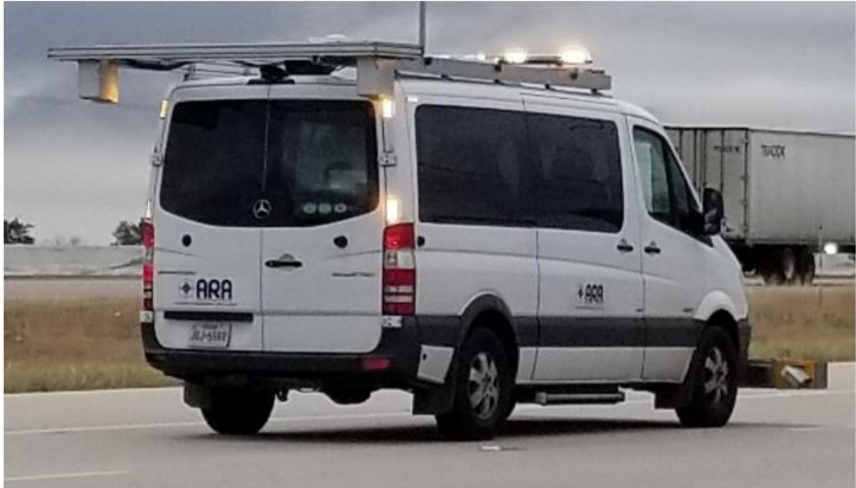
Figure 1 — ARA Multi-Function Vehicle (Equipped with 3-D LCMS).
