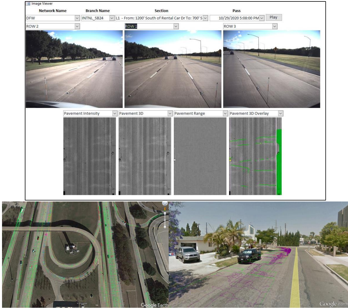
Figure 7 — ARA Right-of-Way Image Viewer and Google Earth Crack Map.
