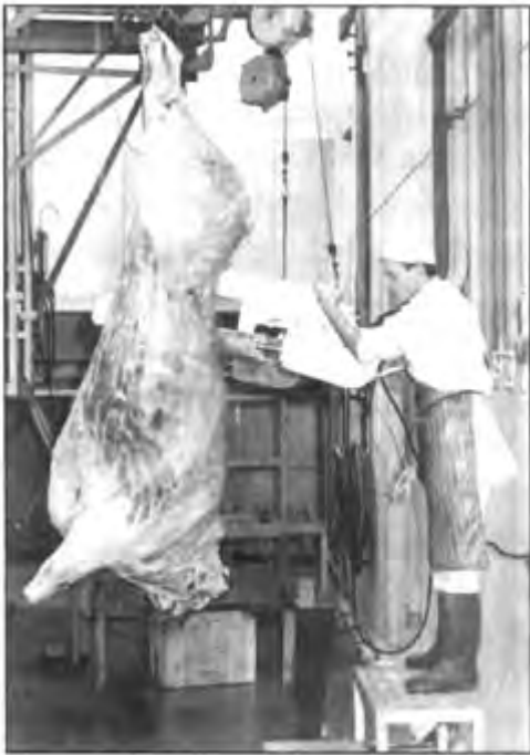
50. Hand-saws are much slower than mechanical saws though they are preferable to cleavers which splinter bones
