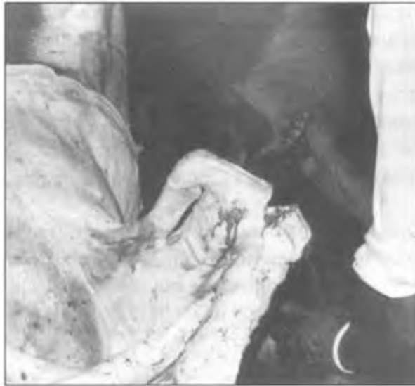
35. Pneumatically operated rotating knives (flayers) speed the removal of the hide from the flanks
