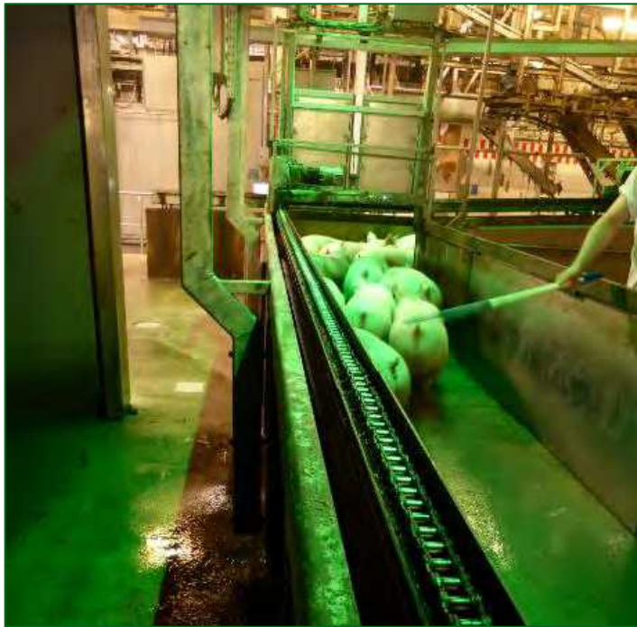
Green lighting was installed at Tönnies to reduce shadows.
