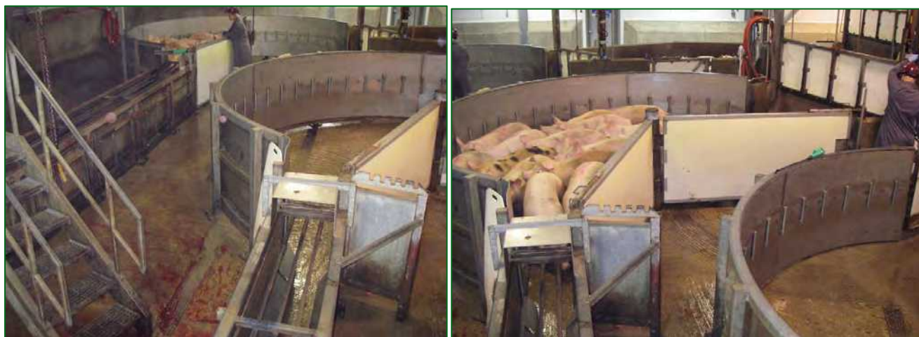
The Corral system. This design works very well according to Temple Grandin. There are however too many pigs in the Corral system on the picture. Temple Grandin recommends to only fill up half of the Corral system with pigs.
