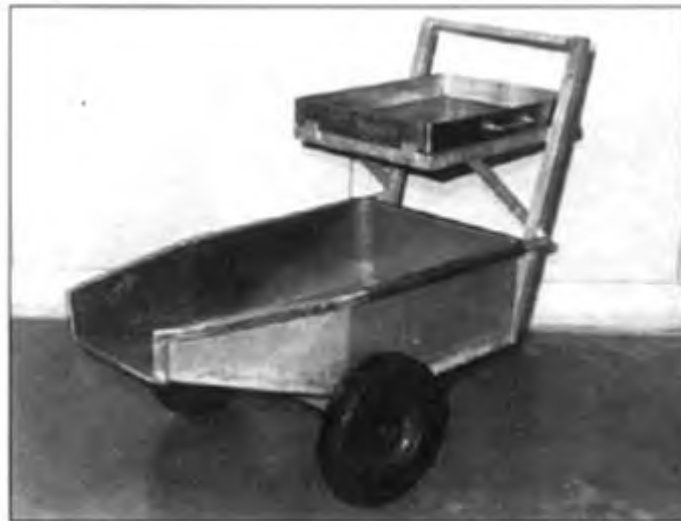
47. A portable cart suitable for catching cattle stomachs and intestines with a separate tray for edible offal such as liver, heart and lungs
