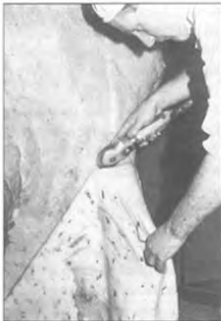
35. Pneumatically operated rotating knives (flayers) speed the removal of the hide from the flanks
