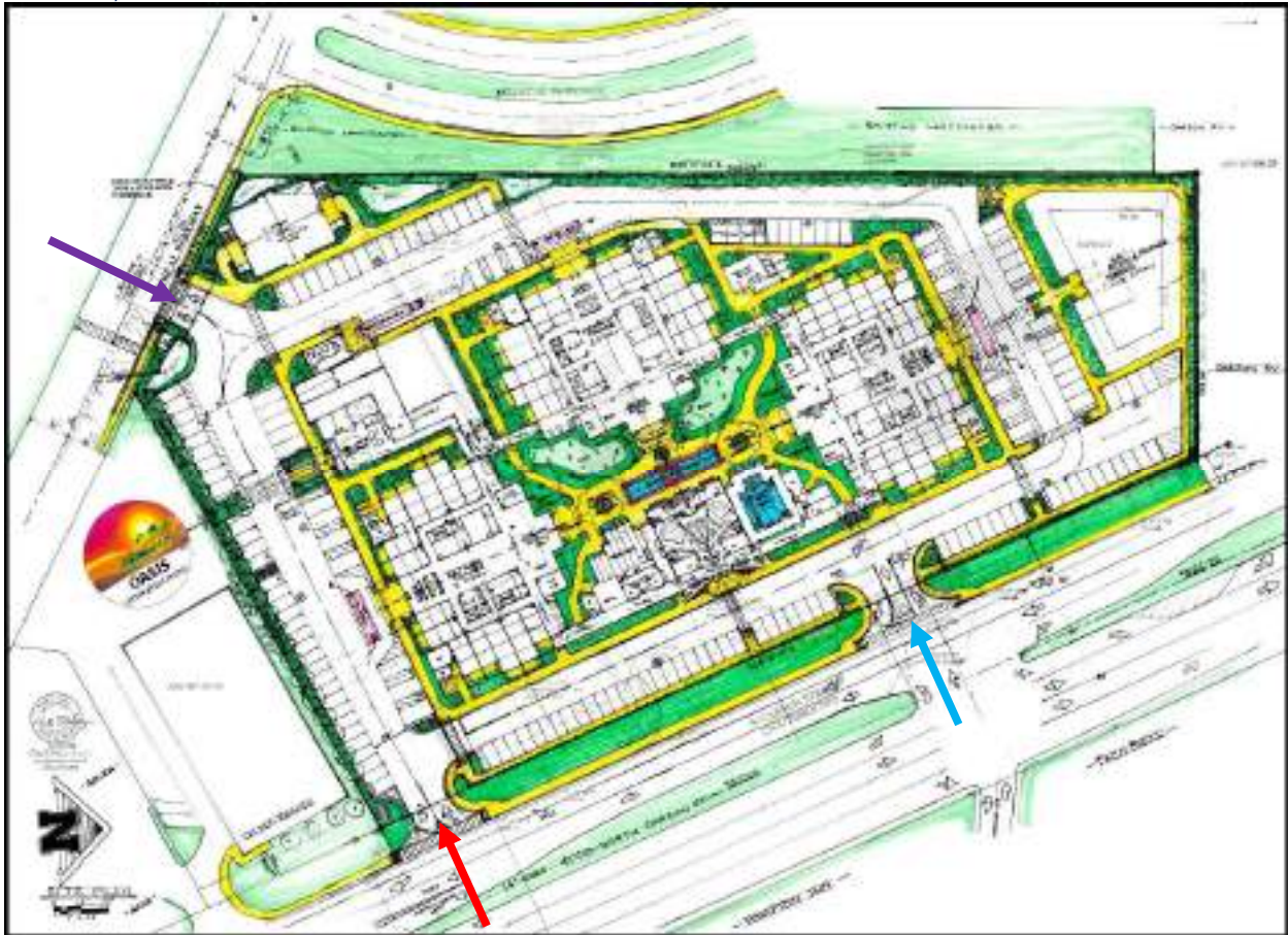
Figure 2 – Conceptual Site Layout of Project. Three access driveways are proposed, with the all direction access driveway for N. Carson Street as a blue arrow, the right in / right out identified as a red arrow, and the Medical Parkway access driveway Identified as a Purple Arrow.
