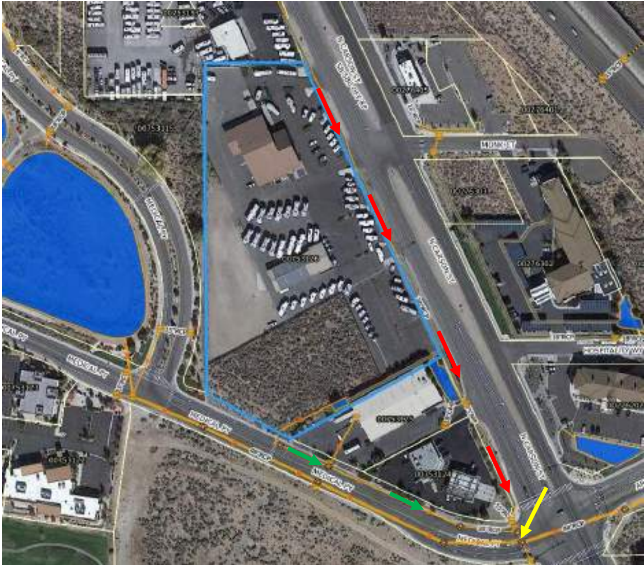
Figure 2 – Overview of Existing Drainage Features on and around the subject parcel. An approximate location of the subject property is shown as a blue outline. Two existing drainage paths exist. There is a drainage path along the east side of the subject property along the west side of N. Carson Street (red arrows), as well as a drainage path on the south side of the property along Medical Pkwy (green arrows). Both drainage paths join up at the yellow arrow where they enter a 48" RCP that heads east along Arrowhead Pkwy. (Imagery from Carson City, MapGeo GIS, courtesy of Carson City Public Works). These are the existing 100 year storm paths for the subject property.
