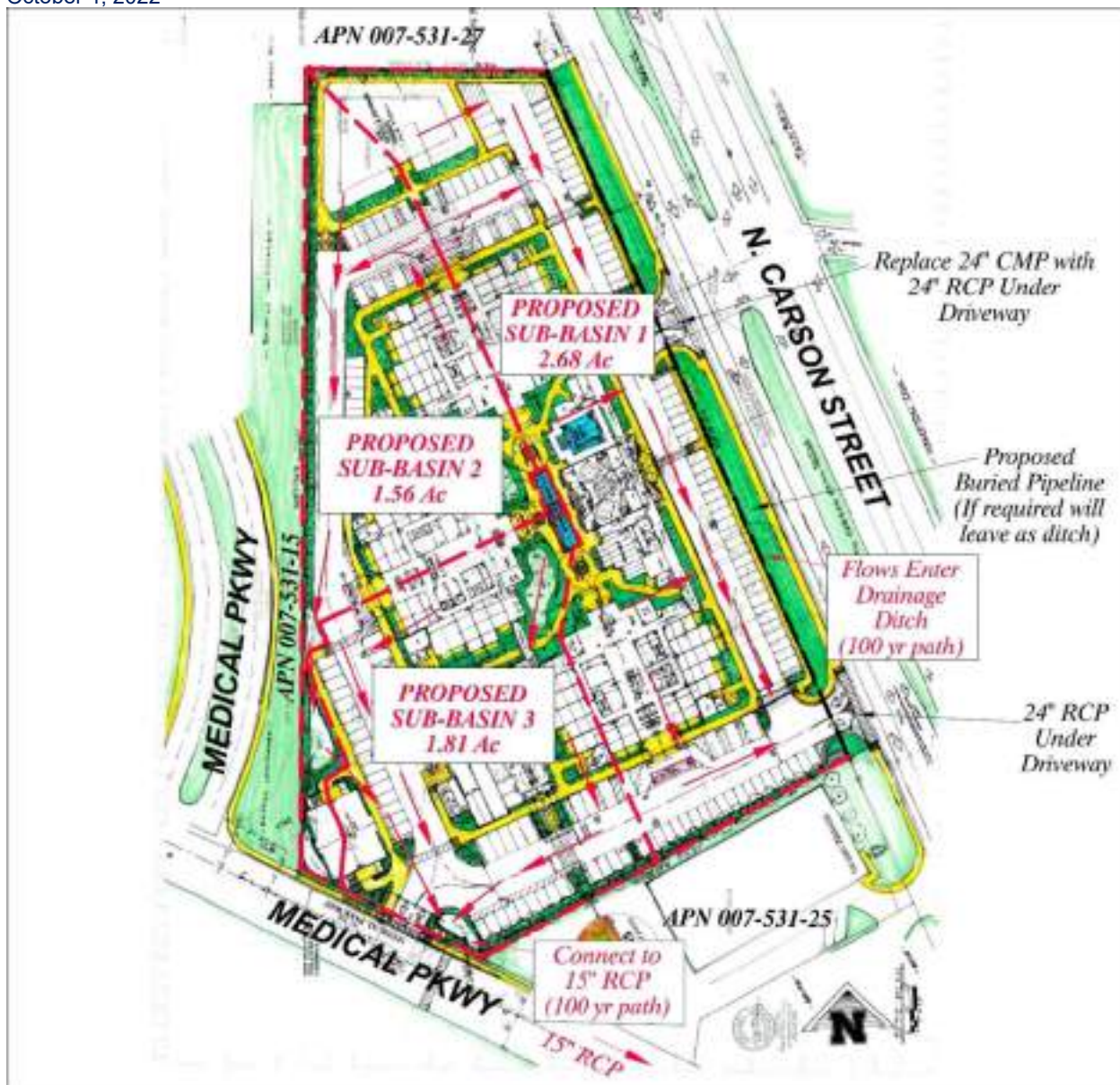
Figure 8 – Overview of Proposed Sub-basins. Three Sub-Basins are evident. Sub-Basin 1 is 2.68 acres in size and drains directly to the drainage ditch on the east side of the property (100 year flowpath) via a 12" buried CMP. Sub-Basin 2 is 1.56 acres in size and flows and drains to a detention basin in the southwest corner of the proposed lot, followed by an overflow to a drainage sump in Sub-Basin 3. Sub-Basin 3 is 1.81 acres in size and flows into a proposed drainage sump in the southern portion of the lot. Here the flows from both Sub-Basin 2 and Sub-Basin 3 will comeingle before entering the 15" RCP pipeline along Medical Pkwy (100 year flowpath).
