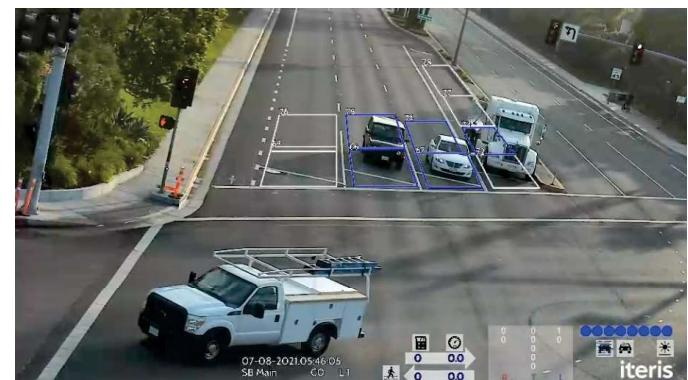
The Vantage Apex sensor enables decision-zone safety functions, collision avoidance and advanced lane-by-lane detection that delivers precise traffic detection and data.
