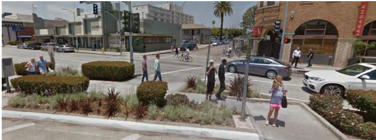
A Pedestrian Island in large intersections helps shorten crossing distances. Source: Google Streetview
