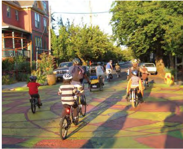
A Painted Intersection, planters, and curb extensions to reinforce that the street is intended for local, low-speed use instead of cut-through vehicle traffic.
