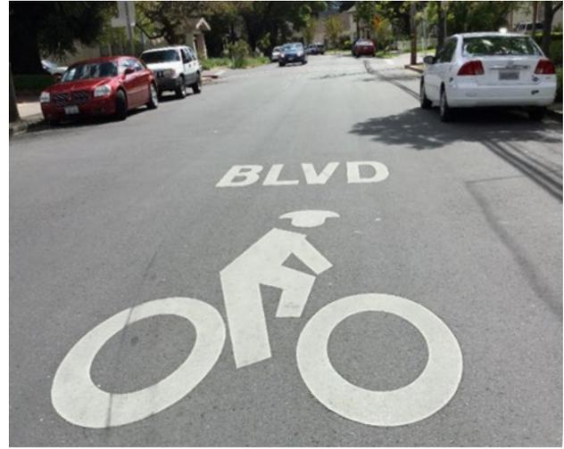
*An example of an large pavement marking to reinforce that the street is a Bike Boulevard.*
