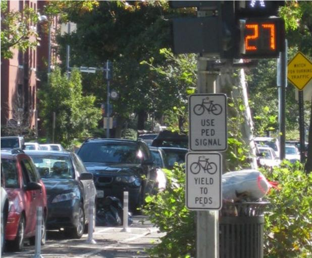
*A bicycle signal head at a signalized crossing creates a protected phase for cyclists to safely navigate an intersection.*
